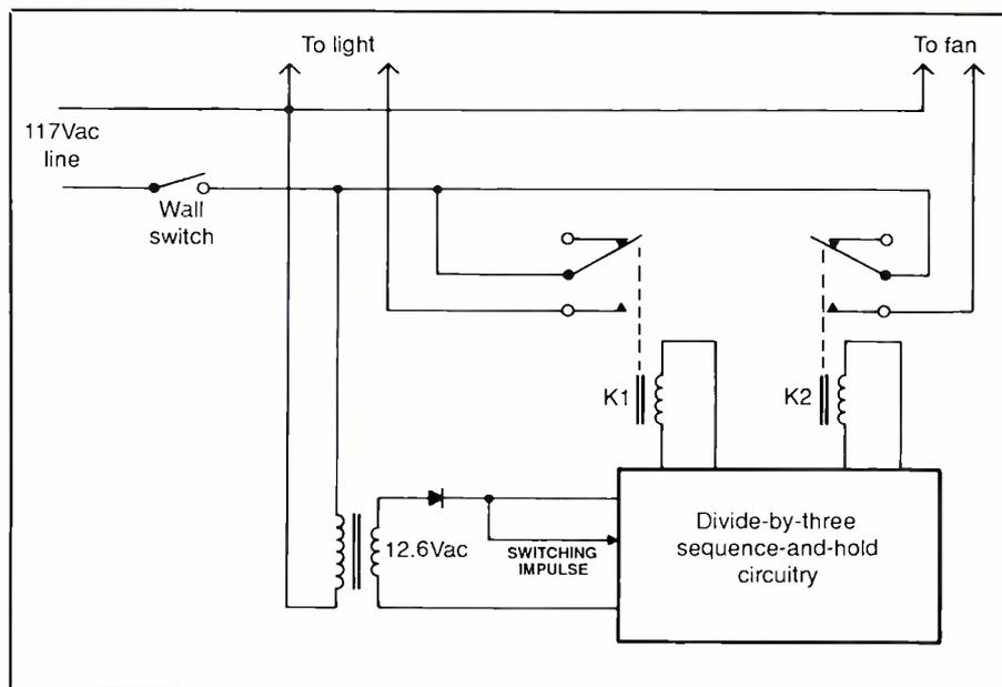
Fig. 1. Simplified diagram of the elements that make up a device that controls two ac-operated electrical devices with a single ac line.
